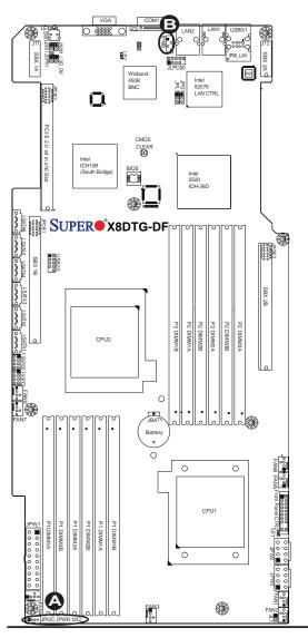
A. PWR I<sup>2</sup>C (SMB) B. IPMB SMB
